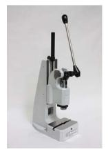
Model No. DIE.D0882.0001 Specimen Size or Difference Between Fixtures 4" gauge length, 1" gauge width, 8" total
