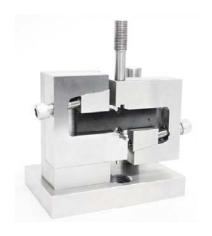
Model No. ASTM.C1292.20 ASTM.D5379.13 Specimen Size or Difference Between Fixtures
